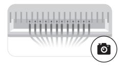
Exposed sprinkler wires with 24VAC could generate an electric shock in wet locations. Please ask your retailer or contractor if sprinkler accessories may be needed.
