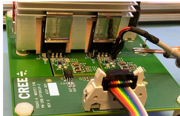
Figure 13. Oscilloscope probe attached
