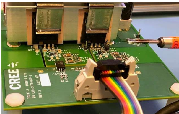
Figure 12. 0.100” pin headers installed
