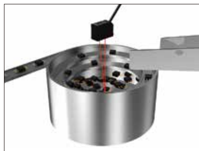
Detecting amount remaining for component feeder (Output 1: Supply starts when amount remaining is small; Output 2: Supply stops when amount remaining is large)
