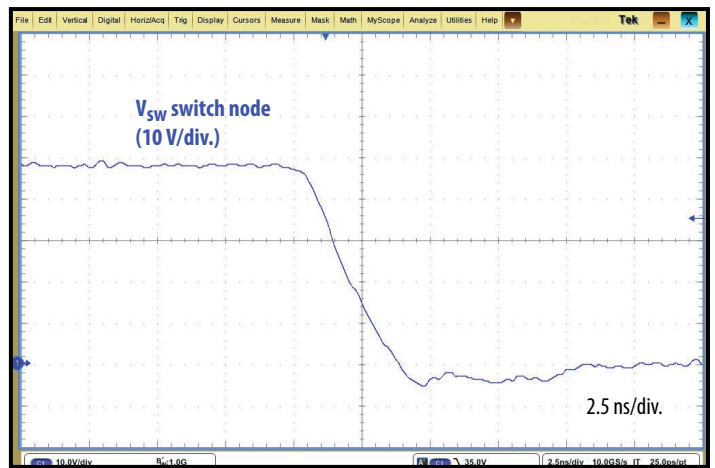
Figure 4: Typical switch node waveforms taken at 48 V IN to 12 V OUT /50 A OUT
