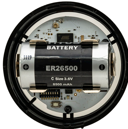
Figure 2. Install the battery as shown
